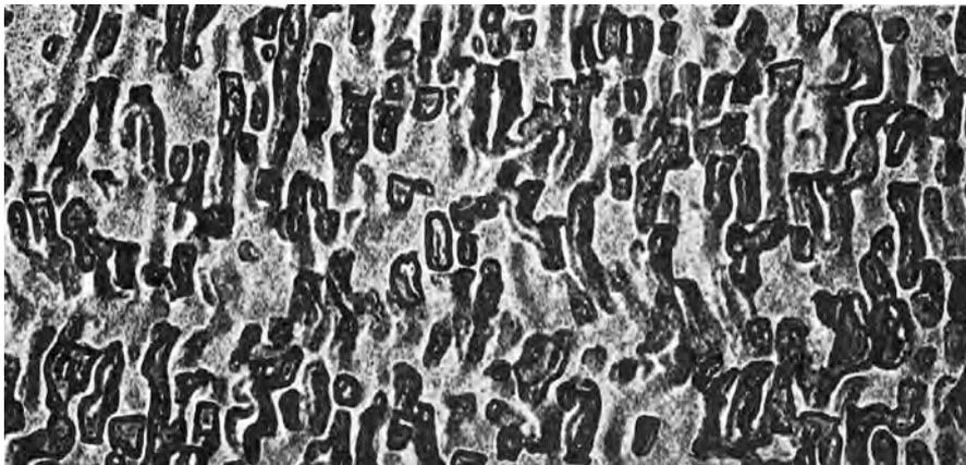
**Figure 32** Microstructure of Alnico V in its optimum state as a permanent magnet. The composition of Alnico V is, by weight percent, 8 Al, 14 Ni, 24 Co, 3 Cu, 51 Fe. As a permanent magnet it is a two-phase system, with fine particles of one phase embedded in the other phase. The precipitation is carried out in a magnetic field, and the particles are oriented with their long axis parallel to the field direction. The width shown is 1.1  $\mu\text{m}$ . (Courtesy of F. E. Luborsky.)
