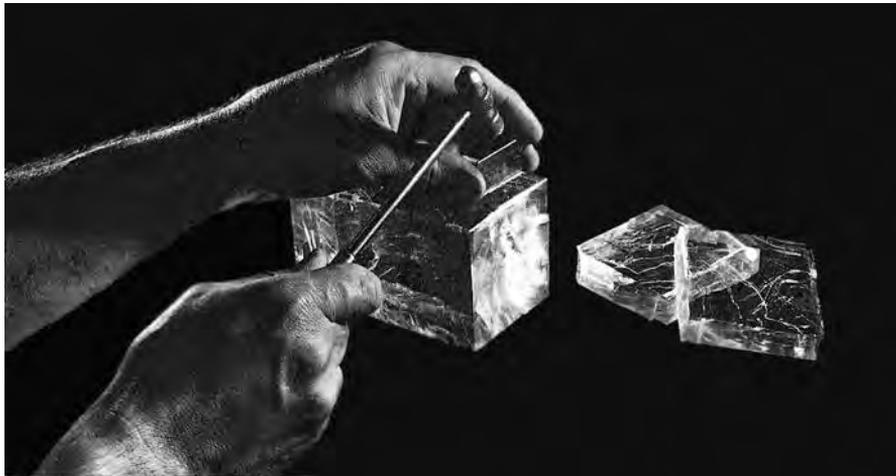
**Figure 1** Relation of the external form of crystals to the form of the elementary building blocks. The building blocks are identical in (a) and (b), but different crystal faces are developed. (c) Cleaving a crystal of rock salt.
