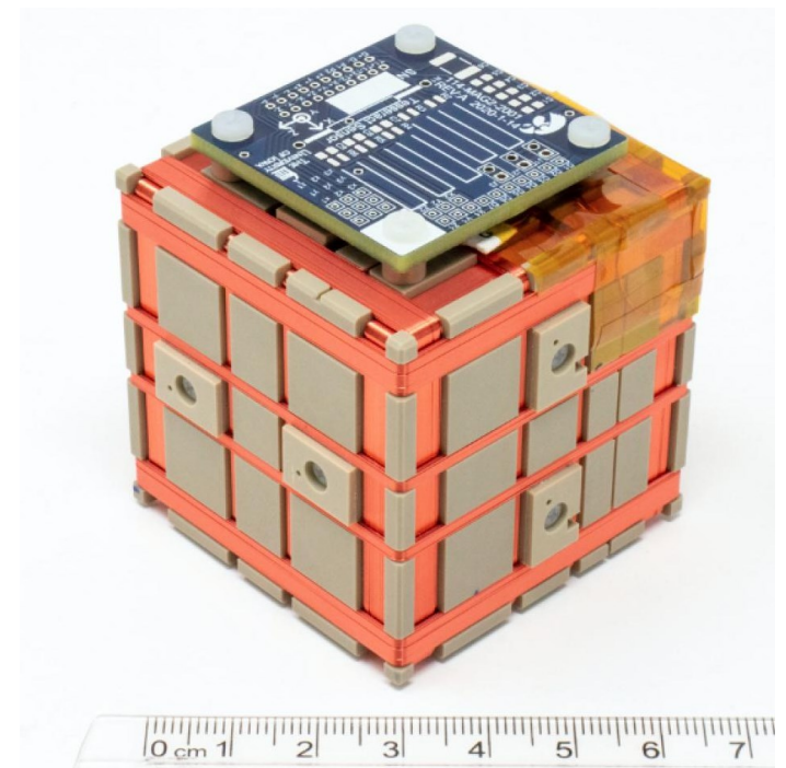
New 'Tesseract' high stability sensor prototype enabled by new styles of fluxgate cores.
